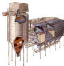
Dry Scrubbing System
